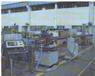
Fig 2. Guide Sleeve Cutting Machine, its control panel and vacuum suction pump
