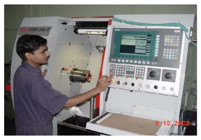
Fig. 1 : R.F. Cavity being machined on a CNC precision lathe
