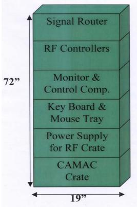
Fig.8 : Control Instrumentation Housing
