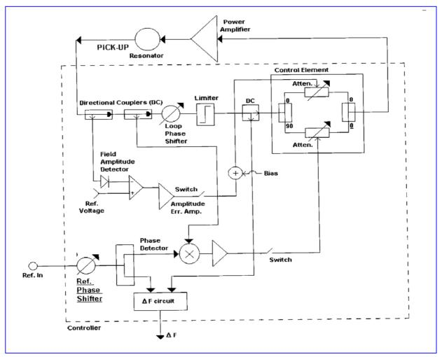
Fig.4 : Resonator Controller
