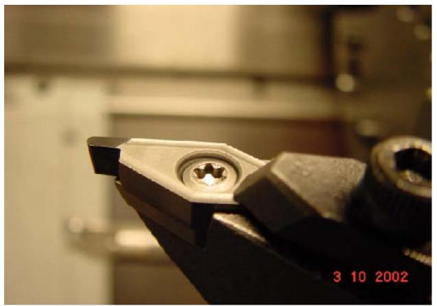
Fig.2 : Customized diamond point cutting tool for machining of cavity profile to achieve surface finish of 0.4µm
