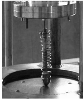
*Fig. 5 : Ball contact point mechanism for damping oscillation*
