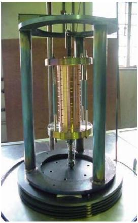
Fig. 4 : Holding fixture along with the 9 cells assembly
