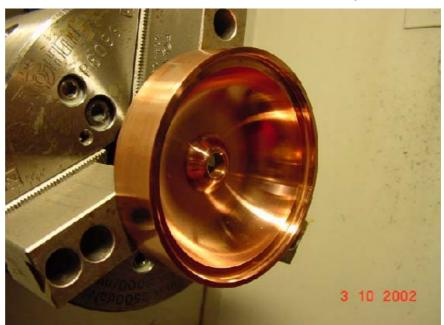
Fig. 6 : A typical brazing groove on CNC lathe under machining
