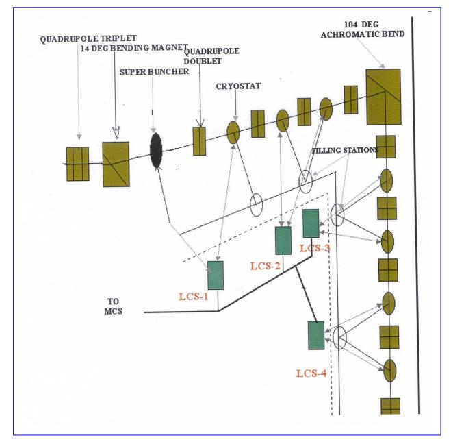
Fig.1 : Layout of the LINAC
