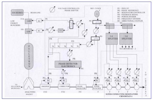
Fig. 3: Block diagram of the RF system for the LINAC booster
