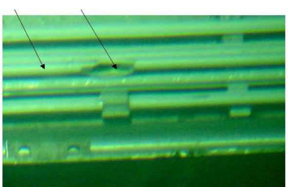
Fig. 6 Underwater PIE of Dhruva fuel cluster at PSIF
