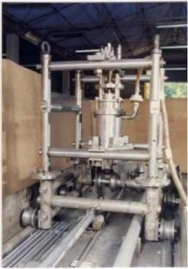
Fig.3 Buggy with cutting mechanism
