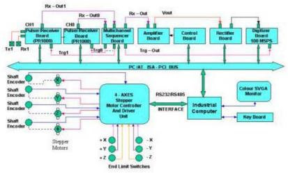
Fig. 4 Schematic block diagram of ULTIMA-100M System
