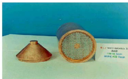
Nb-Ti multi filamentary billet assembly developed at AFD, BARC. It shall produce a 3 km single length superconducting wire of 1.3 mm dia. Fig. 1 Multi-filamentary billet assembly developed at AFD, BARC
