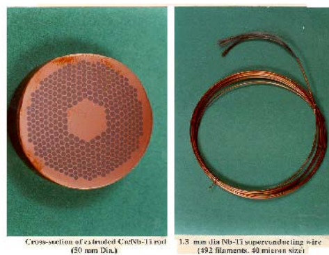
Cross-section of extruded Cu/Nb-Nb-Ti rod (50 mm Dia.) 1.3 mm dia Nb-Ti superconducting wire (492 filaments, 40 micron size) Fig. 2 Cross-section of extruded Cu/Nb/Nb-Ti rod (left) and 1.3 mm dia Nb-Ti superconducting wire containing 492 filaments, each of 40 micron cross-section.
