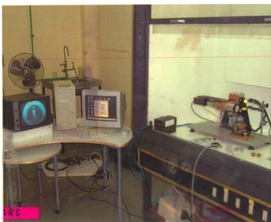
Fig. 2 Laser welding set-up inside a fume hood.
