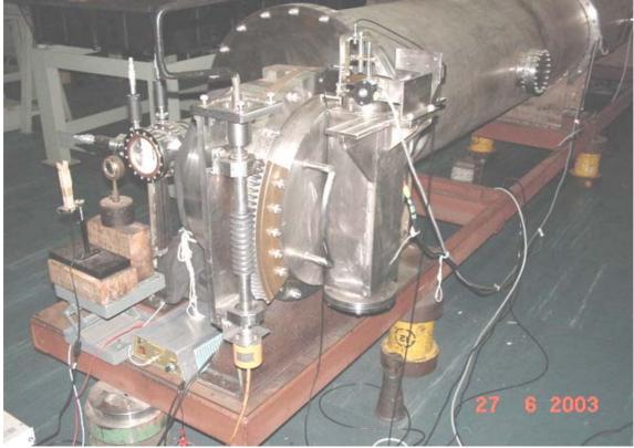
Scanning mechanism end of spectrometer
