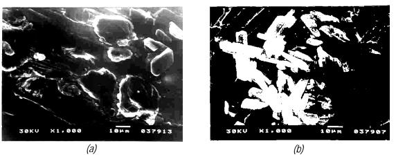
Fig. 1 SEM micrograph of (a) DCS-10 and (b) DCS-20 powders
