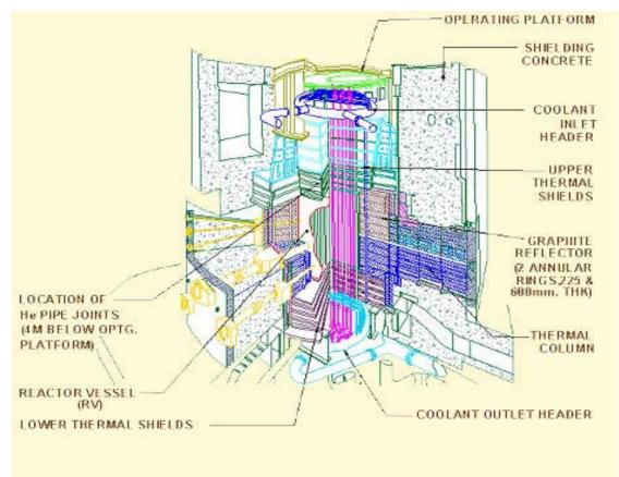
CIRUS reactor structure cross section
