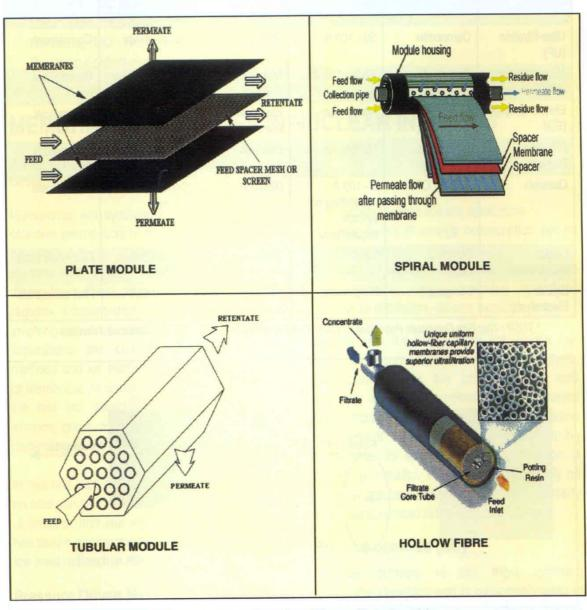
Fig. 2: Different configurations of Reverse Osmosis modules
