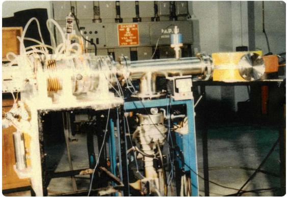
Fig. 1 A close up view of the Duoplasmatron Ion Source
