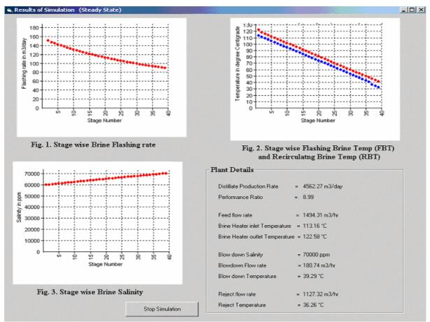
Fig. 4 Final Steady State simulation result form
