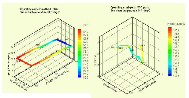
Fig. 8. Operating envelope of the MSF Plant generated by the simulator MSFSIM
