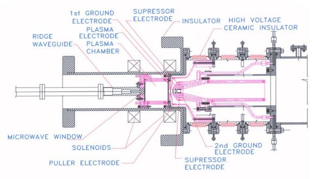
Fig. 5 Schematic of the 50 keV, 50 mA ECR Proton Ion Source
