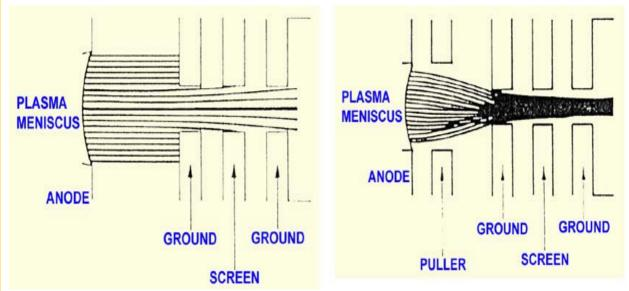
Fig. 6 Transmission of the beam through the Pentode Extraction Geometry
