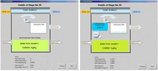
Fig. 3 Details of a Non- flashing stage and a Flashing stage
