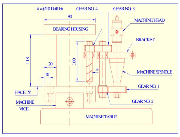
Fig.2 Schematic diagram of Counter Boring Attachment
