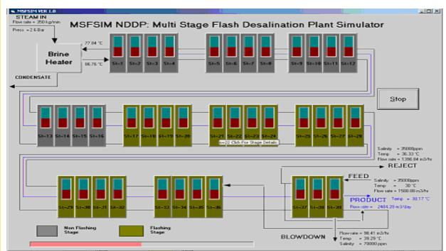
Fig. 2 Main form during Steady State simulation
