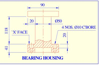
Fig.1: Schematic drawing of Bearing Housing
