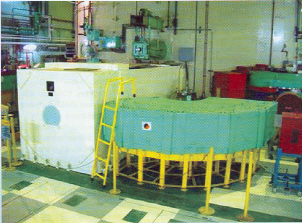
Fig. 10 : Focusing crystal-based diffractometer
