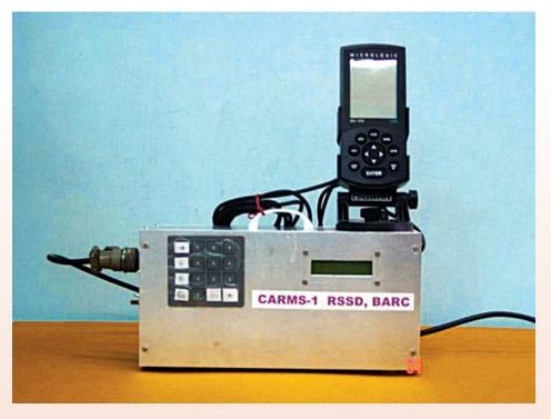
Fig. 9: Compact Aerial Radiation Monitoring System (CARMS) for quick assessment of radiological impact using UAVs
