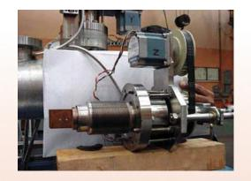
Fig. 2: Slit jaw assembly
