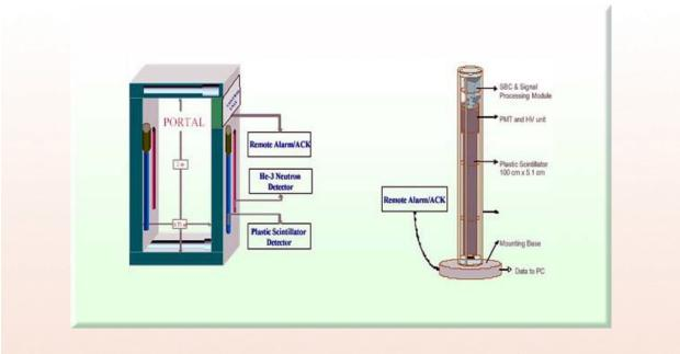
Fig. 10: Portal Monitor and Limb/Pole Monitors developed in BARC for the detection of illegal movement of radioactive materials (Gamma/Neutron)
