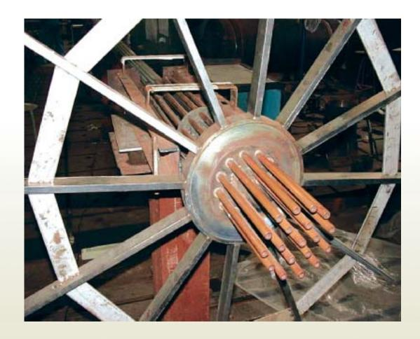
Fig.1: Fuel rod cluster ready for insertion into the channel
