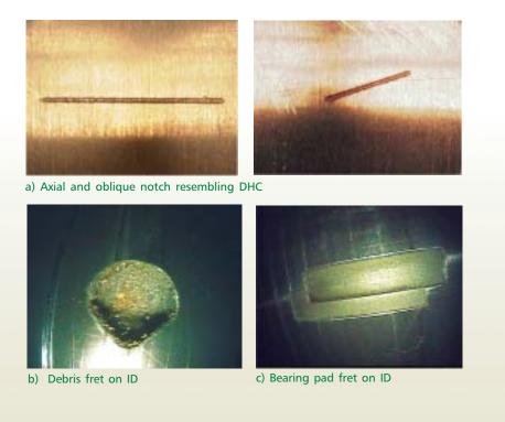
Fig. 4 : Simulated flaws in pressure tube samples
