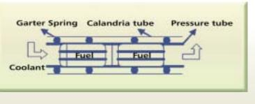
Fig. 1: Simplified sketch of coolant channel
