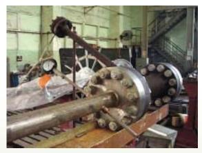
Fig.4: FRCS channel assembly under hydro-testing
