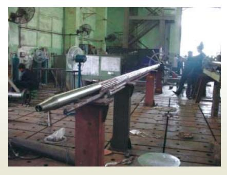
Fig 2: SS tube plate end of fuel rod cluster
