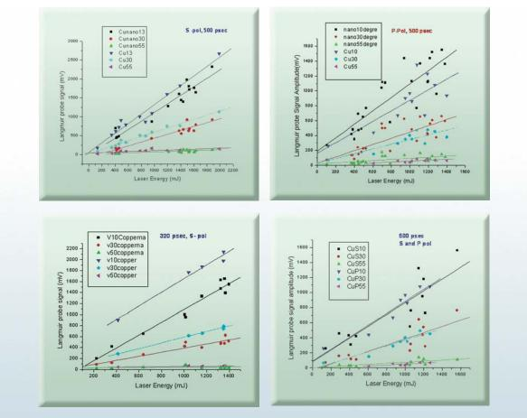
Fig. 11: Scaling of ion densities and ion velocities with laser pulse energy for two polarization measured by set three of Langmuir probes placed at various angles.
