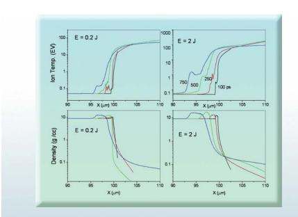
Fig. 8: Spatial profiles of ion temperature and density for laser energy 0.2 Joule and 2 Joules
