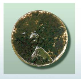
Fig. 2: Biomass collected from fouled pipeline
