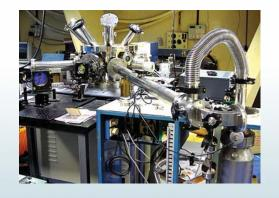
Fig. 7a: Vacuum chamber: outside view
