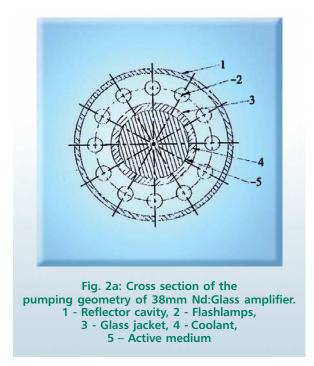
efficiency, low cost and easy availability. Xenon flash lamps convert 40 to 60% of the electrical input energy into radiation, in the 0.2 to  $1.0\mu$ m region, which contain most of the major absorption bands of Nd:Glass [4]. Pumping efficiency becomes poor in large diameter rods, due to non-uniform absorption of pump radiation, leading to a spatially varying gain profile as shown in Fig. 2b.
