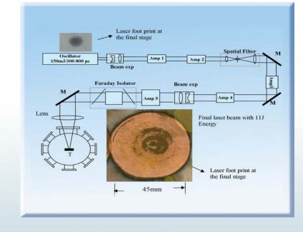
Fig.1a: 10J/300-800 psec laser chain: schematic
