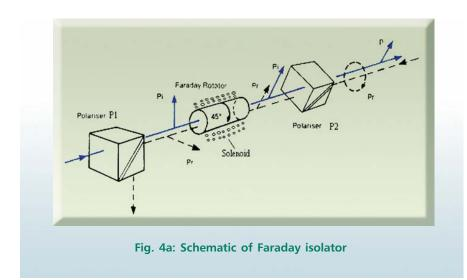
The extinction (ratio of input to back reflected laser intensity) at the centre of the Faraday isolator is found to be 270: 1 and the total transmission loss for input laser measured in the Faraday isolator is about 15 % which is admissible in high power laser systems. The laser pulse exiting from the Faraday isolator has a high peak to background contrast of about 10<sup>4</sup>, which is extremely important for laser-plasma experiments.
