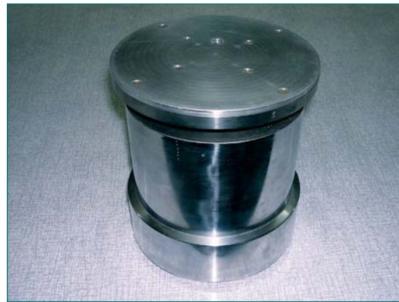
Fig. 2 : TMAC tool compatible with 540 MWe Fuelling Machine
