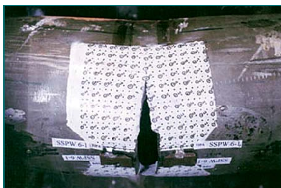
Fig. 25: Pipe weld of 168 mm OD
