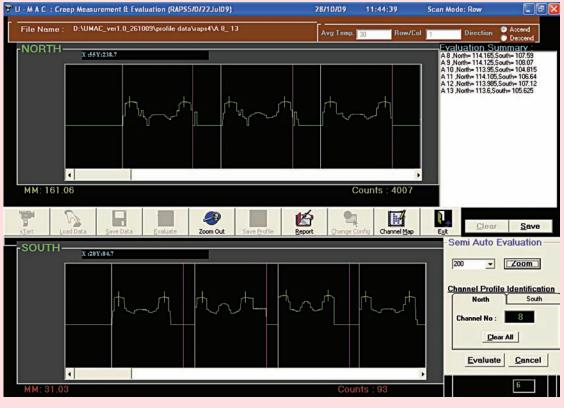
Fig 6: Measurement & Evaluation of channel profile
