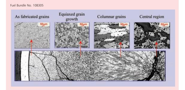
Fig. 18 Restructuring in fuel occurs due to a steep temperature gradient from the centre to the periphery of the fuel. Boundaries of the microstructural regions in an irradiated  $UO_2$  fuel can be used as markers for estimation of fuel centre temperature attained during operation.
