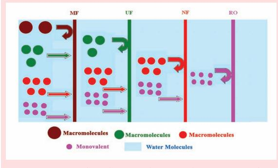
Fig.1: Membrane processes (MF-microfiltration, UF-Ultrafiltration, NF- nanofiltration, RO-Reverse Osmosis)
