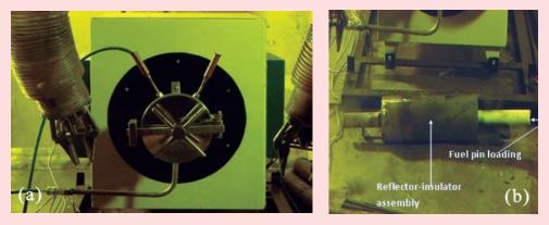
Fig. 13: Furnace used for ballooning studies on irradiated fuel
