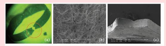
Fig. 12: Deformation behaviour of clad after burnup level of above 15000 MWd/tU at 583 K showing (a) significant level of ductility (b) failure by void formation in the central portion of specimen followed by (c) localized shearing at 45° to the loading direction.
