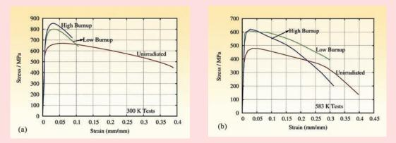
Fig. 11: Circumferential tensile deformation behaviour of low and high burnup fuel pin claddings, (a) at ambient temperature (300 K) showing irradiation hardening and reduction in clad ductility and (b) at 583 K showing significant increase in clad ductility at elevated temperature.
