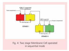
The generator system operated in this mode has greater convenience and is being used for generation of carrier free <sup>90</sup>Y on regular basis.
