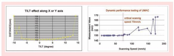
Fig 2: Experimental qualification of UMAC sensor under operating condition of FM tilt and FM scanning speed
