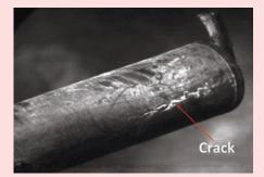
Fig. 3e : Crack on the cladding of an outer fuel pin from bundle no. 108305
