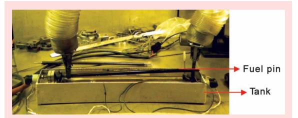
Fig. 6 : Ultrasonic immersion scanner for PHWR fuel pins. Motors fitted on both ends of the tank are used to translate the ultrasonic probe along the length of the fuel element and also to rotate the fuel to enable helical scanning of the fuel element cladding. The system can also be used for the ultrasonic inspection of end plug welds.
