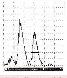
Fig. 5d: Signal from a defective weld with partial fusion
