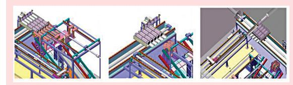
(a): Pusher-I Sub-assembly (b) X-Table Sub-assembly (c) Pusher-II Sub-assembly
