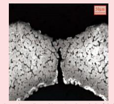
Fig. 13d Metallographic section through the failed region of the cladding. The grain boundary cavities indicate that the primary cause for failure is thermal creep.
