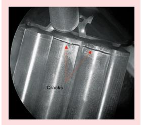
Fig. 3b End cap weld cracks observed in PHWR fuel bundle no. 54505.
