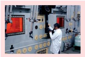
Fig. 3a: Wall periscope for visual examination in hot cells facility.
