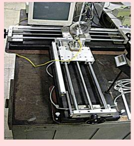
Fig 5: Sensor Calibration Manipulator
