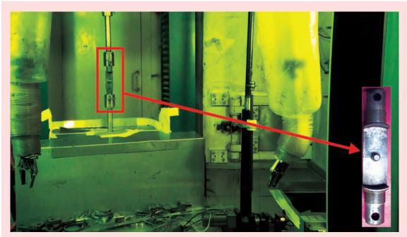
Fig. 10: Screw driven universal testing machine inside the hot cell and the ring tension test grip set (right inset).
