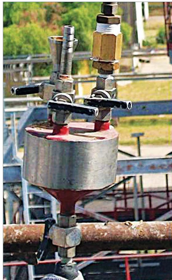
Fig. 2: A typical tracer injection system
