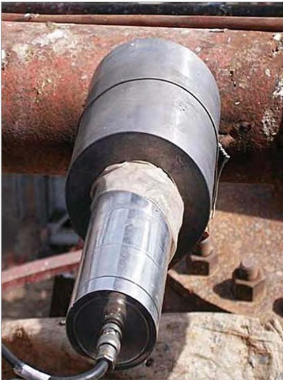
Fig. 3: Collimated scintillation detector
