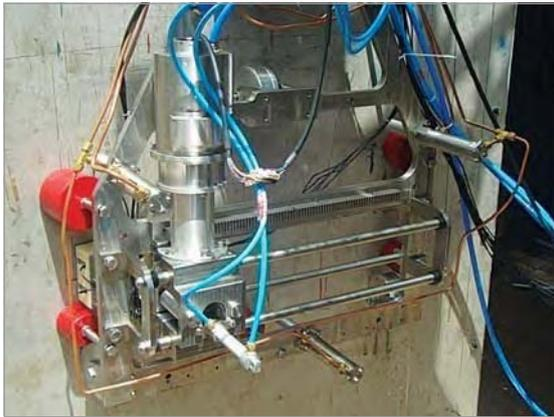
Fig. 11(b): WIM with cross travel and probe holder
