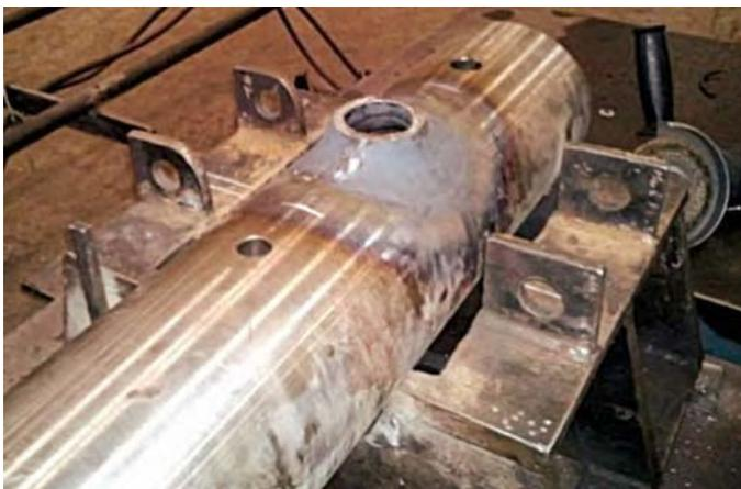
Fig. 14: Component with nozzle pulled-out
