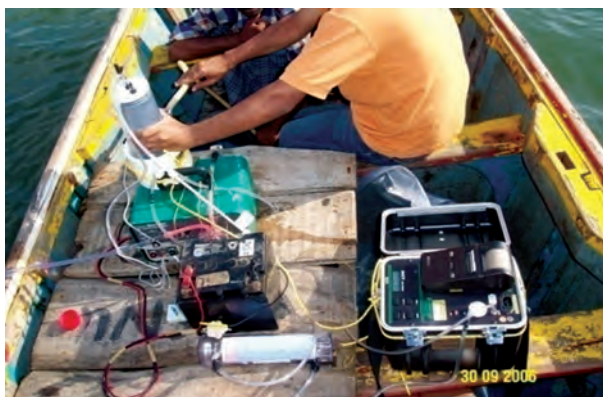
Radon Meter (RAD7) Natural ^{222}\text{Rn} in water samples
