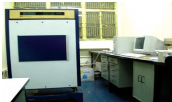
Liquid Scintillation Counter for measurement of ^3\text{H} , ^{14}\text{C}
