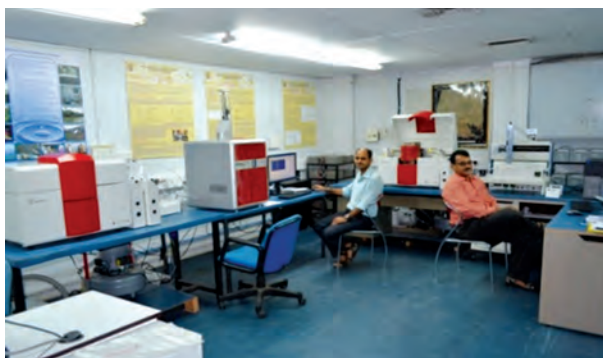
Isotope Ratio Mass Spectrometer for measurement of ^2\text{H} , ^{18}\text{O} , ^{13}\text{C} , ^{15}\text{N} and ^{34}\text{S} .
