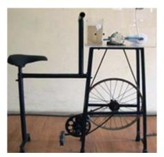
Fig. 7: Foot operated RO/UF units
