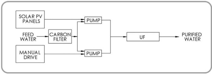
Fig. 3: Process Schematic of the UF System
