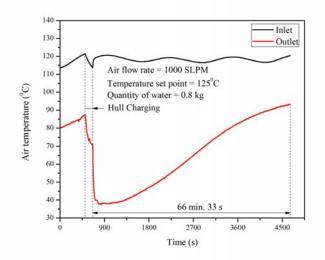
Fig. 3: Air temperature at inlet and outlet of hull dryer as a function of time
