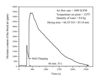
Fig. 4: Time variation of moisture content in the bleed air
