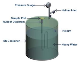
Fig.1. Design of stainless steel container for storage of high purity heavy water reference standard
