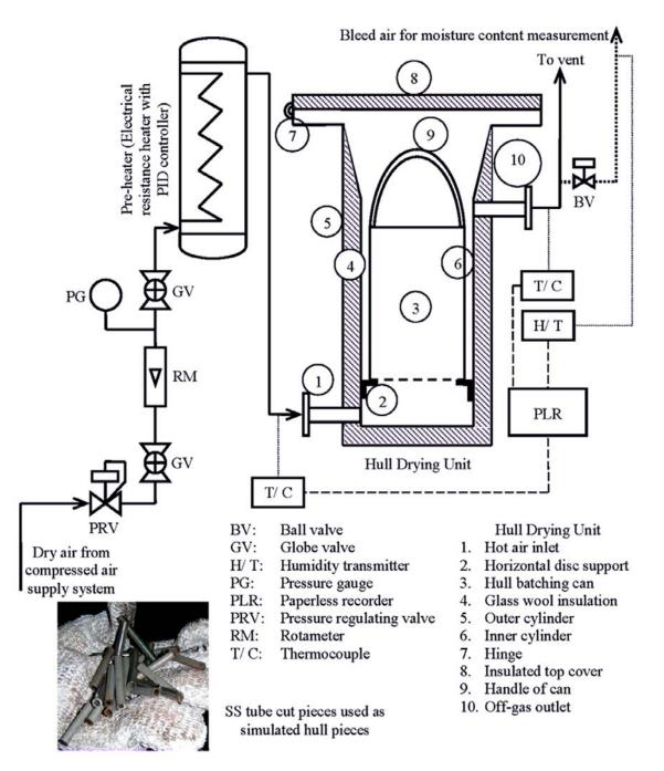
Fig 1: Schematic sketch of experimental setup
