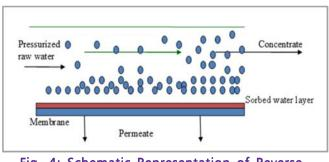
Fig. 4: Schematic Representation of Reverse Osmosis
