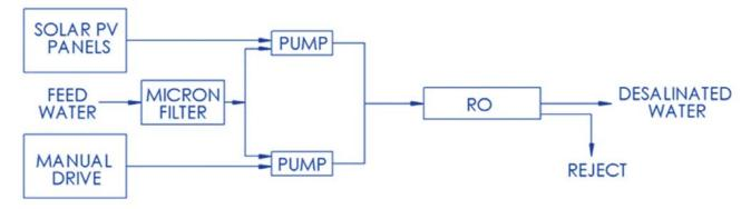
Fig. 5: Process Schematic of the RO System
