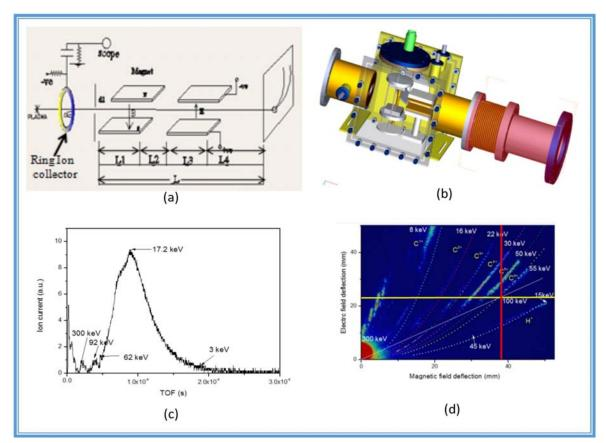
Fig. 2: (a) Schematic of Thomson parabola ion spectrometer (b) Design of TPS (c) Ion collector signal and (d) Thomson parabola record of the graphite plasma.
