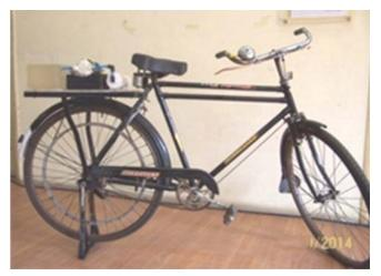
Fig. 8: Bicycle-mounted, foot/pedal operated RO / UF units
