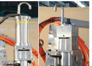
Fig. 8: Remotely removable motor couplings and impact head for manual override
