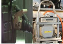
Fig. 7: Modified electrical connector for remote operations
