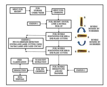
Fig. 2 Flow chart of Head-End Operations for PRTRF
