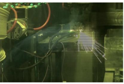
Fig. 10: Laser dismantling of irradiated Thoria bundle inside hot cell
