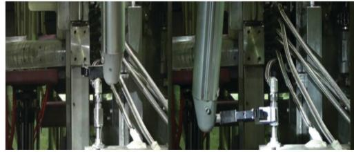
Fig. 9: Hydraulic connectors for decoupling and coupling operations using MSM
