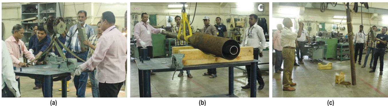
Hands-on training given to the trainees to handle the material using EOT Crane at TRP Workshop, Tarapur (a) Rigging practice (b) Moving pipe in horizontal direction in close proximity (c) Uprighting of pipe
