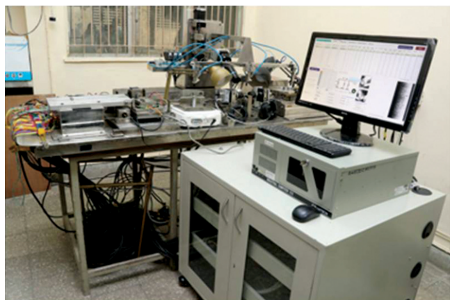
Fig. 4: (a) Pellet imaging set up.
