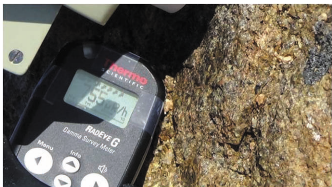
Fig.17: Highest radiation dose rate on a rock in Betts Island
