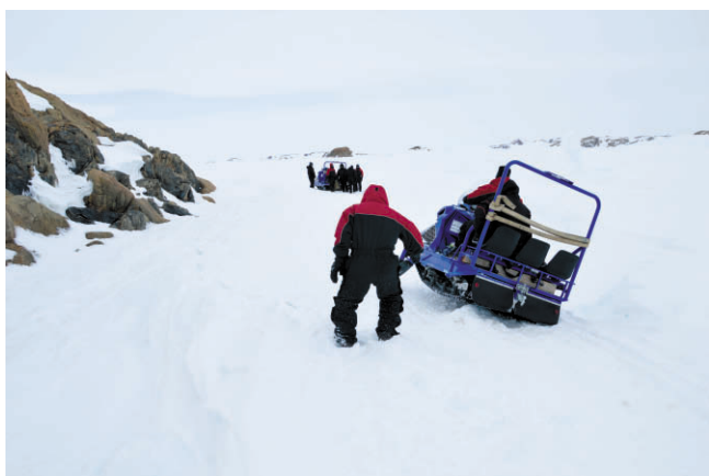
Fig. 12: Skidoo mishap caused by onset of melting of snow
