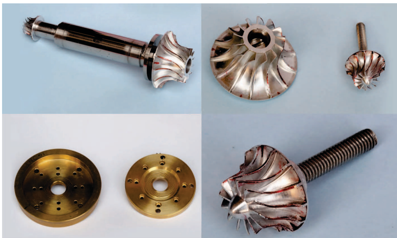
Fig. 2. Photographs of the turboexpander wheels used in the developed system
