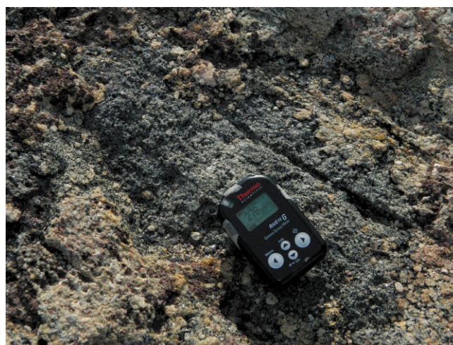
Fig.9: Radiation survey showing hotspots with radiation levels of about 200 \mu\text{R/h}
