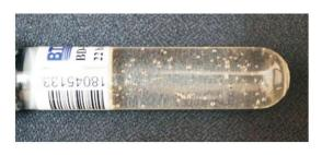
Fig. 8: Neutron generated bubbles in a bubble detector from deuterium target in D-D mode
