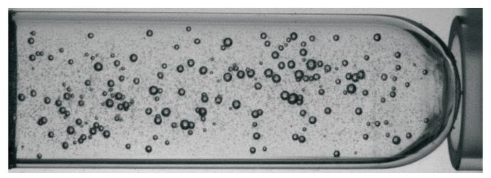
Neutron generated bubbles seen through detector reader
