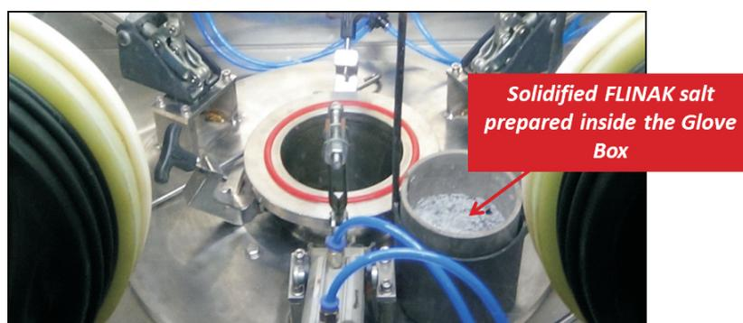
Fig. 4: FLiNaK salt prepared in MSCT Facility
