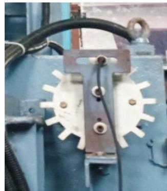
**Fig. 9: Tooth type proximity sensor**
