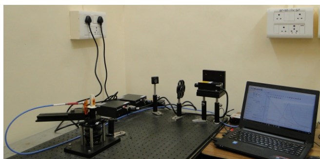
Fig.2: Optical setup for angle-resolved emission studies.
