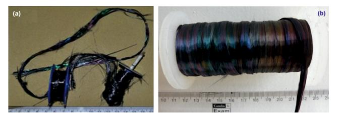
Fig.4: Reel to reel produced SiC fibre. (a) almost fully converted SiC fibre (5 m length), (b) SiC coated carbon fibre (>20 m length).
