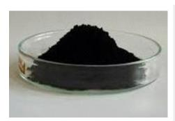
Graphene oxide used in preparation M30 concrete
