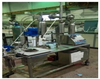
Fig.1: Autoclave for synthesis of PCS.
