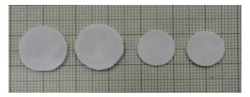
Fig.8: LAGP glass ceramics disks of various dimensions (Diameter: 12mm, Thickness: 0.7mm).
