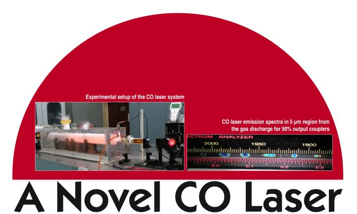
Lasing action in 5 µm region occurring from CO molecules formed inherently in a CO<sub>2</sub>-N<sub>2</sub>-He gas discharge lead to applications in spectroscopy & material processing
