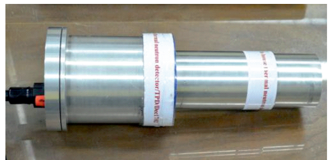
Fig.10: A USB based handheld thermal neutron detector employing Lil:Eu 2+ single crystal.
