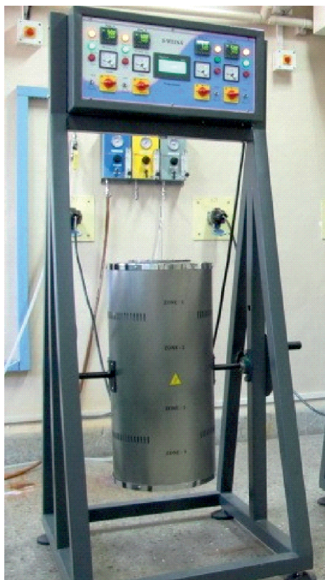
Fig.1: A typical Bridgman Crystal Growth Furnace.
