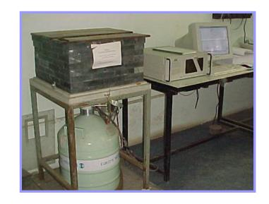
Characteristic gamma radiations emitted from radio nuclides are measured using HPGe detector. Intensity of gamma radiations are proportional to the concentration of radio nuclides
