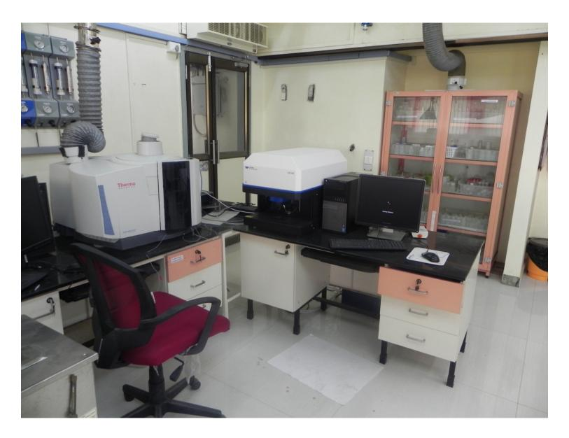
Inductively coupled plasma—optical emission spectrometer coupled with laser ablation system: For analysis of trace elements in metals and rock samples.
