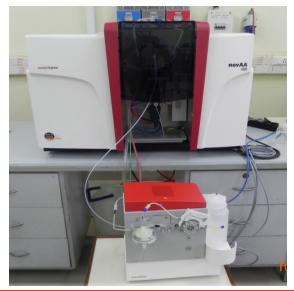
Key Components of novAA800F Source: Hollow Cathode Lamp Atomiser: Air Acetylene Flame and Hydride generation attachment Background correction: D<sub>2</sub> Detector: Solid state
