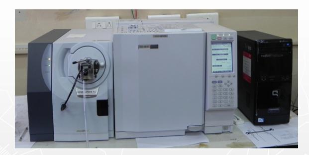
**Applications** : Identification and quantification of volatile and semi volatile organic compounds in complex mixtures eg. pesticides in food, beverages, organic pollutants in water, environmental samples, etc. Determination of molecular weight, structural determination of unknown organic compounds.
