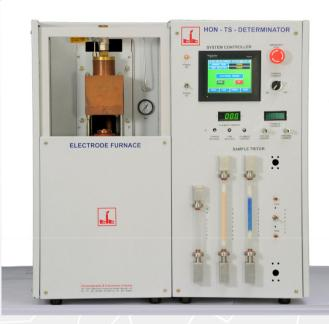
**Principle:** The equipment is based on inert gas fusion technique. The sample is heated to a high temperature in a graphite crucible with tin flux under inert atmosphere. Hydrogen is detected by thermal conductivity detector
