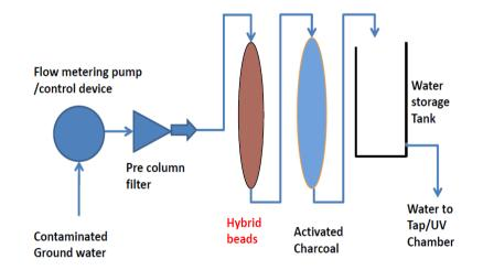
Sorption capacity of different developed materials Process flow diagram for community based online operation
