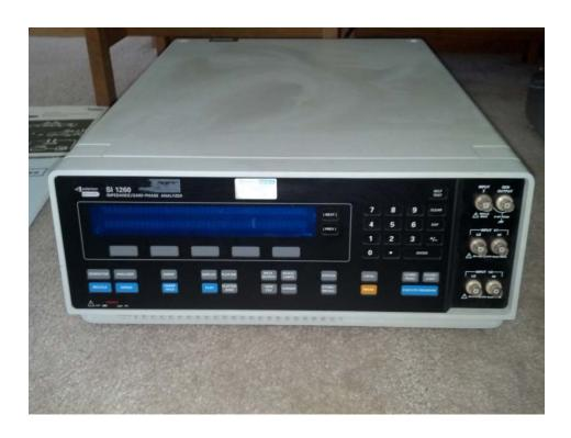
The instrument measures impedance of solid and liquid samples in the frequency range 1  $\mu$ Hz to 32 MHz. A high temperature cell has been attached to this instrument to measure the conductivity, dielectric constant of solid samples up to 800 °C.
