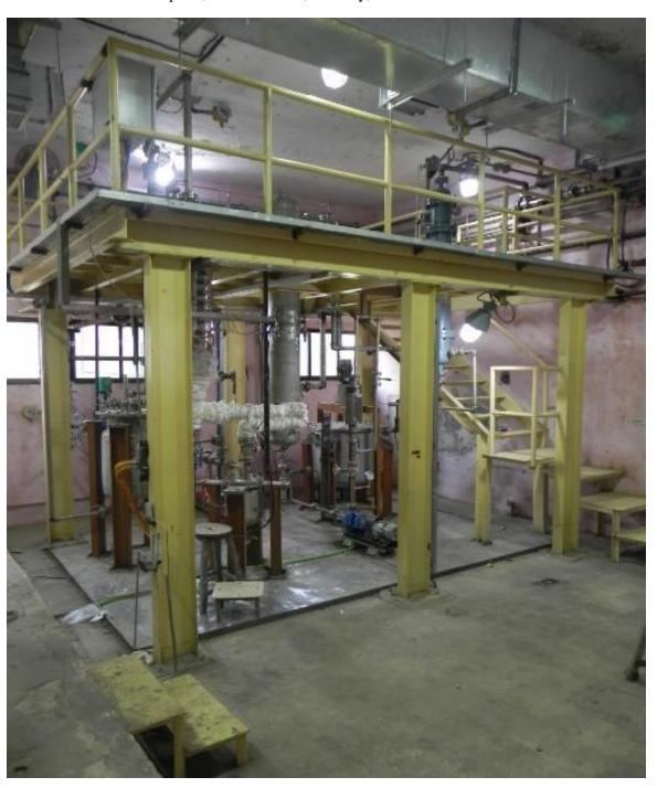
Fig. 1. Experimental setup of FCVD process
