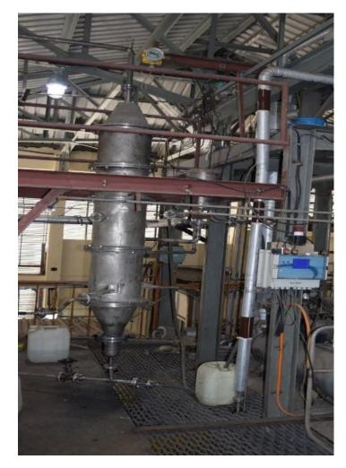
Fig.4 Multi-stage circulating fluidized bed (MSCFB) for organic vapour adsorption, recovery and reuse.
