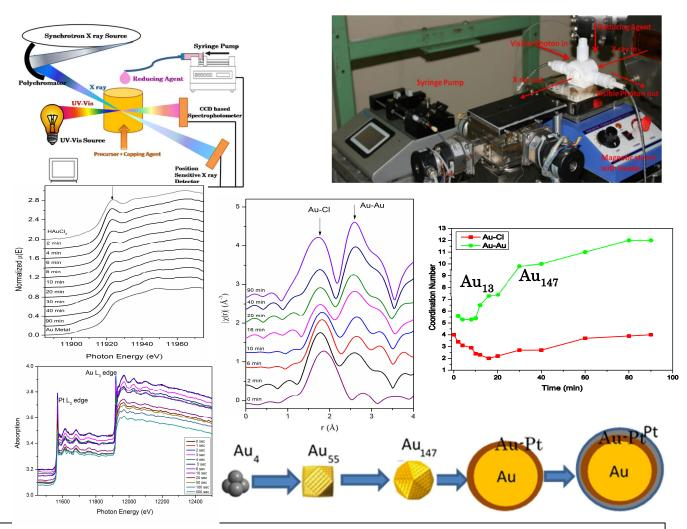
• Facility for *in-situ* XAS measurements on growth of nanoparticles (2016)
