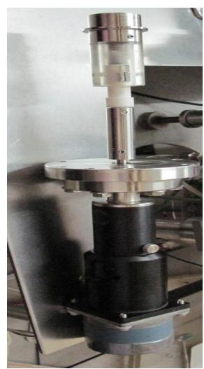
Sample Probe attached to a Stepper Motor
