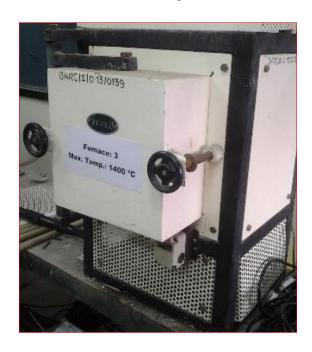
Electrical heating furnace with ambient condition suitable for preparing oxide sample
