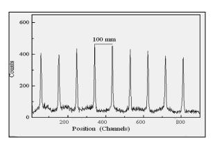
Position spectrum of a <sup>3</sup>He PSD with slit-3 and 10 cm spacing
