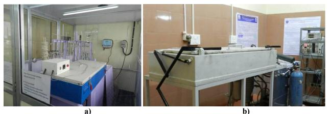
a) System for generation and distillation of BF<sub>3</sub> gas from CaF<sub>2</sub>(BF<sub>3</sub>) complex
