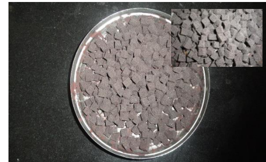
(\text{Fe,Cr})_2\text{O}_3 foam catalyst granules
