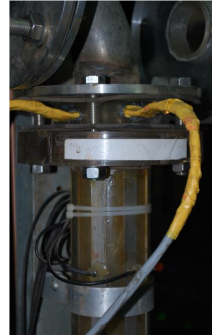
8X8 WMS Installed in Two-phase Air-Water Set-up
