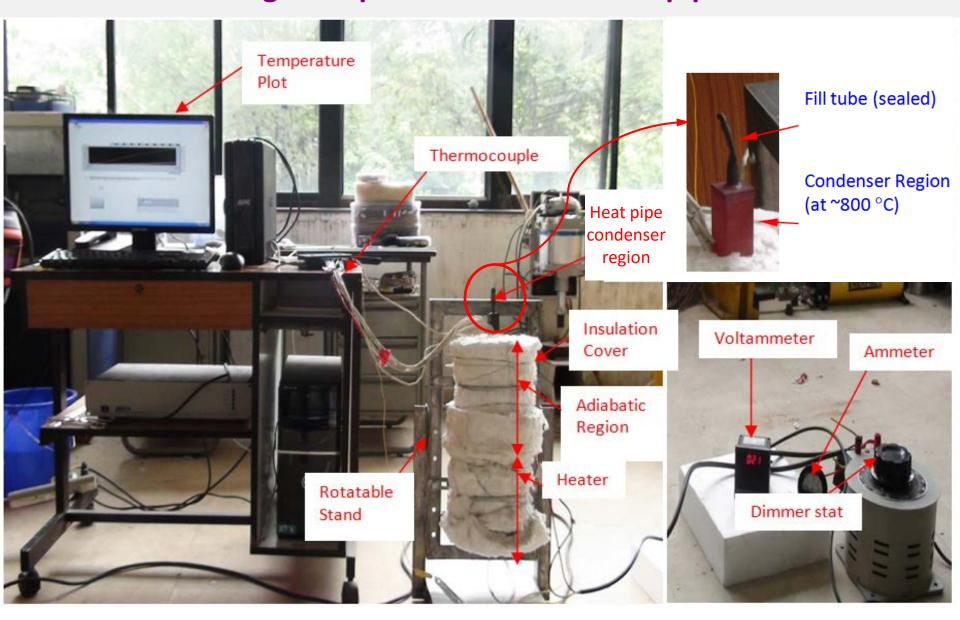
Design, fabrication of a sodium heat pipe and its operation upto 800 °C has been successfully demonstrated.
