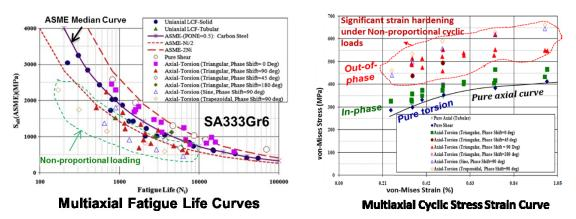
The above figures show that under multiaxial non-proportional loading the fatigue tests have showed significant strain hardening as well as reduction in the fatigue life when compared with corresponding uniaxial results.
