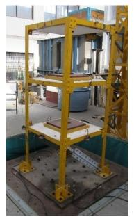
Shake Table Testing of Steel Frame with BRB
