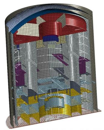
Finite Element Model of AHWR Reactor Building
