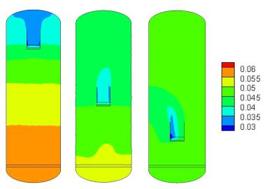
Hydrogen Mole Fraction Contours for three different recombiner Location
