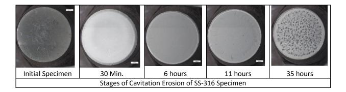
A Cavitation Erosion Test Facility has been developed and qualified as per ASTM G32. The test facility is being utilized for evaluating cavitation-erosion resistance of various stainless steels and coatings.
