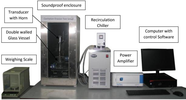
Photograph of Cavitation-Erosion Test Facility
