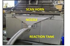
Reaction tank and nozzle in beam room
