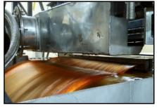
Effluent flow under electron beam
