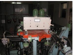
Seismic testing of Control panel
