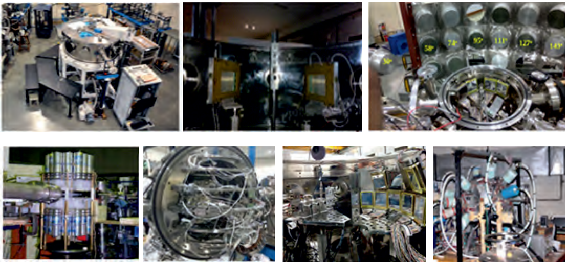
Fig. 6: Experimental facilities set up at PLF a) 1.5m diameter Multipurpose scattering chamber for reaction studies b) High granularity large solid angle strip detector array for charge particle detection c) Liquid scintillator array for neutron measurements d) \text{BaF}_2 array for high energy gamma rays measurements e) \text{CsI} array for light charge particle detection f) MWPC detectors for fission measurements g) High efficiency, high resolution Indian National Gamma Array (IGNA) for gamma ray measurements
