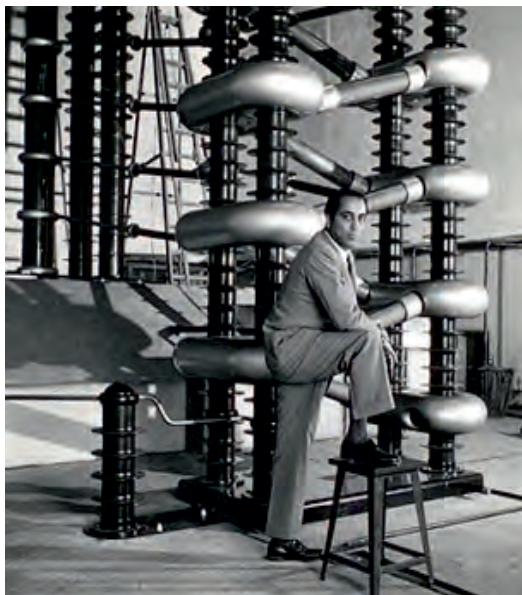
Fig. 2: 1 MV Cockcroft-Walton Accelerator (Cascade Generator) at TIFR, in 1953
